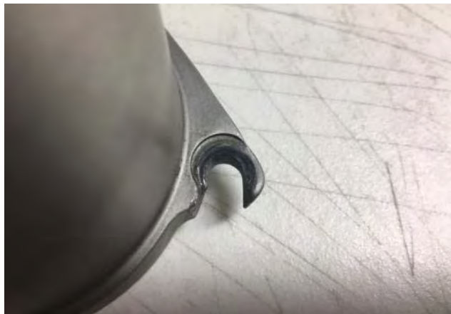
The fuel filter bowl has two lobes with slots (180 degrees apart). These slots engage the attachment studs.
