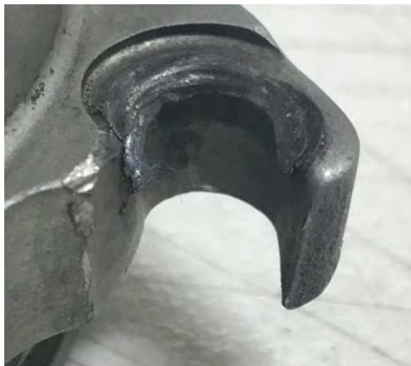
The fuel filter bowl has two lobes with slots (180 degrees apart). These slots engage the attachment studs.
