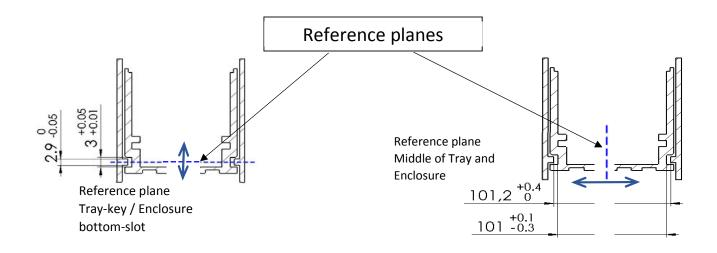
The tolerances for connector positions in back plate of enclosure and tray should are not being taking into account.
