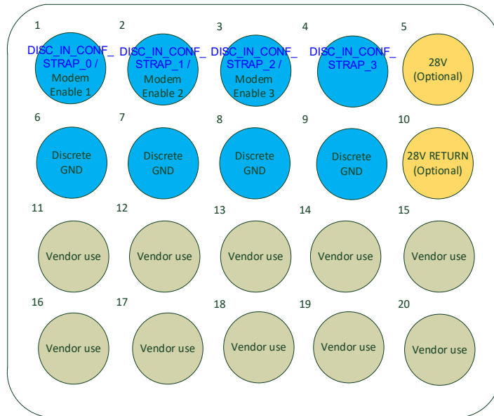
Figure 17-x – CCM/CWAP J3 (pins)
