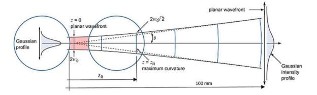
The surface of the receiving lens needs to be positioned (z) well within the Rayleigh distance  $(z_R)$  and preferably within the Near-field zone ( $z < z_R$ ). For multimode, the Rayleigh distance  $z_R$  is typically less than 50mm and the Near-field is less than 25 mm. For single mode  $z_R$  is less than 10 mm and the Near-field is within a few mm's. The divergence angle of the far-field beam (at 100 mm) will not really contribute any useful information.
