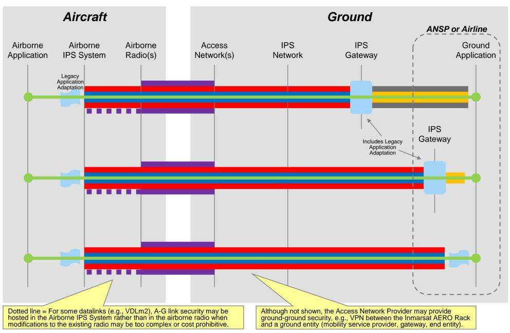
Color Legend: Legacy Application IPS Transport Legacy Transport IPS E2E Security Ground-Ground Security Air-Ground Link Security
