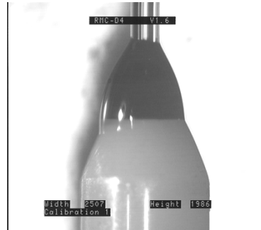
Figure 5-9 – Excessive Epoxy on Ferrule End Face
