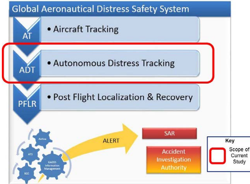
Figure 1: Scope of ADT Report Requirements and Architecture Studies with Respect to ICAO GADSS Scope (ref GADSS CONOPS Ver 6)
