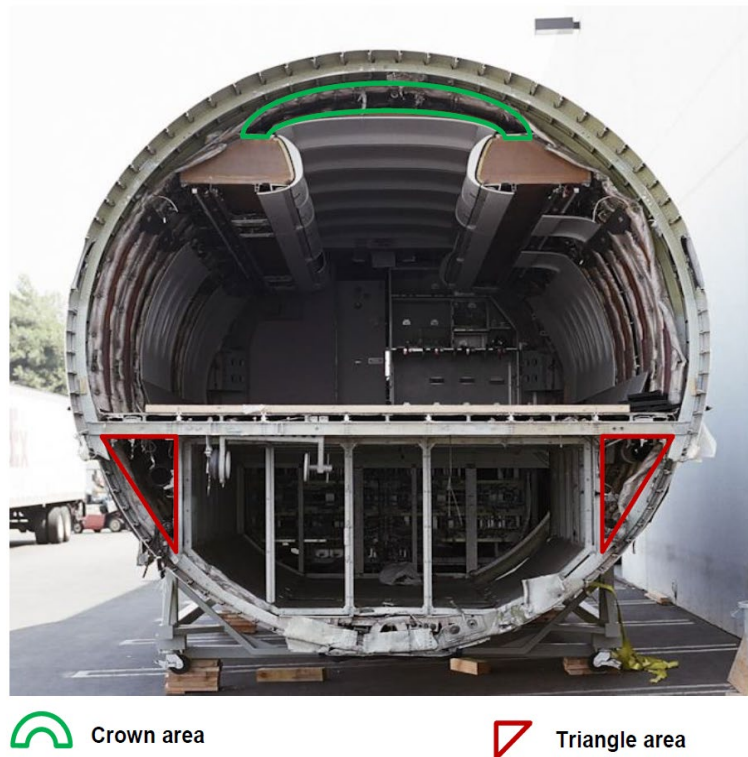
Figure 7-1 – Potential Remote Radio Unit Location Areas
